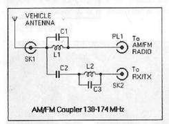
The  $5/8\lambda$  antenna is fitted with RG58U coaxial cable, which goes to the SO239 socket on the coupler itself. The standing wave ratio should be checked and any adjustments required made by cutting the whip shorter, little by little, until the best SWR has been achieved.
